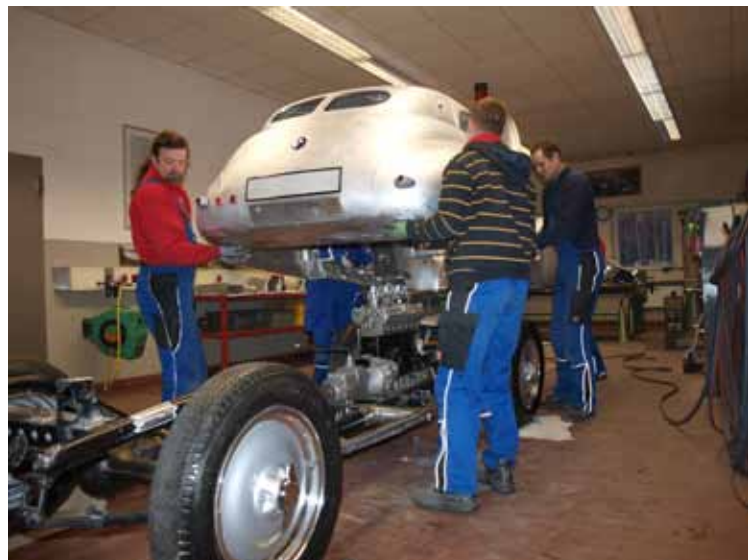
Interim trial fitting of the body on the tubular frame.
